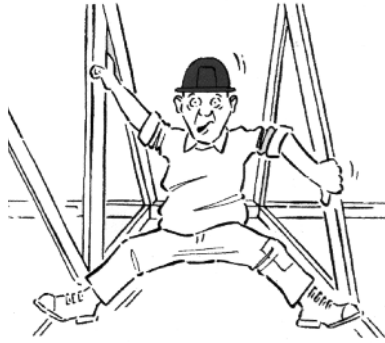
Trusses DO need bracing
